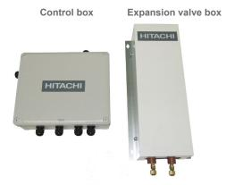
The DX-Interface series 2 is used to allow the connection of third-party manufacturer units to Hitachi outdoor units, which enables the control of their direct expansion coil (for R410a) following Hitachi control logic. Typical applications are air handling units (AHU), air curtains and units similar to standard indoor units (standard indoor units understood as cooling/ heating indoor air treatment units for room conditioning).
