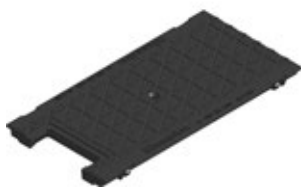
Ductile iron solid cover with opening for cables, (SW 128/49 mm), black, KTL-coated class C 250, locked, 0,5 m
