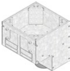
Drain box for type 100, 150 with paveable cover
