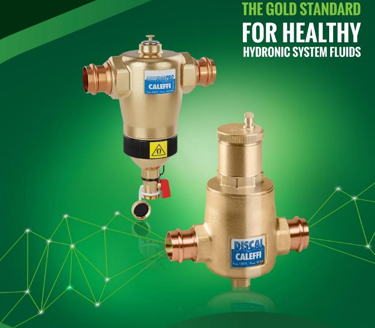
The **DISCAL®** air separator and **DIRTMAG PRO®** dirt separator duo ensures maximum protection and efficiency in hydronic systems. The DISCAL high efficiency air separator features a large, low-flow zone, coalescing element and automatic air vent to minimize corrosion formation. The DIRTMAG's magnetic technology and particle mesh removes both ferrous and non-ferrous debris helping to keep expensive heat exchangers and ECM circulators running smoothly. **CALEFFI GUARANTEED.**
