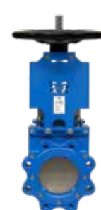
Series 702/20 Knife gate valve with handwheel and rising stem DN50-1200 PN10 Ductile iron Options: • handwheel and non-rising stem • chainwheel • electric or pneumatic actuator • lever
