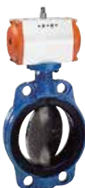
Series 75/31 Butterfly valve Centric with fixed liner Semi lug type DN50-300 PN10/16 Ductile iron Options: • full lug type • various actuators
