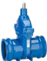
Series 01/80 Gate valve with "Euro" socket ends for uPVC-pipes DN40-400 PN16 Ductile iron
