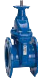
Series 15/42 Flanged gate valve for electric actuator Face-to-face DIN F4 DN40-400 PN10/16 Ductile iron Options: • face-to-face DIN F5 • hydraulic/pneumatic actuator • NBR wedge
