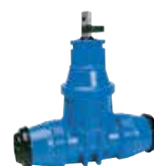
Series 16/54 Service connection valve with tensile socket ends for PE pipes DN25-50 PN16 POM (Polyoxymethylene) Options: • ductile iron
