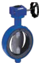
Series 75/10 Butterfly valve Centric with fixed liner Wafer type DN40-1400 PN10/16 Ductile iron
