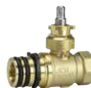
Series 103/31 Angle service connection valve with Supa Lock™ spigot/push-in socket end DN32 PN16 Ductile iron
