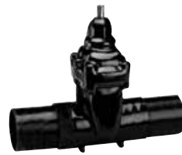
Series 46/70 Gate valve with long spigot ends DN50-600 PN16 Cast steel GP240GH External PUR coating
