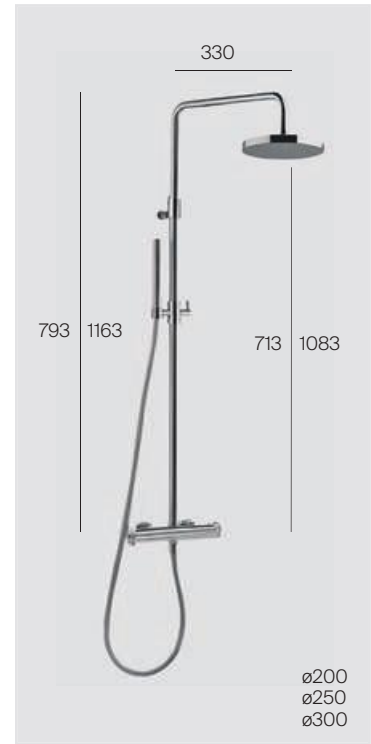
FP389 Columna telescópica termostato 2 duchas Telescopic column thermostatic 2 showers Colonne télescopique thermostatique 2 douches
