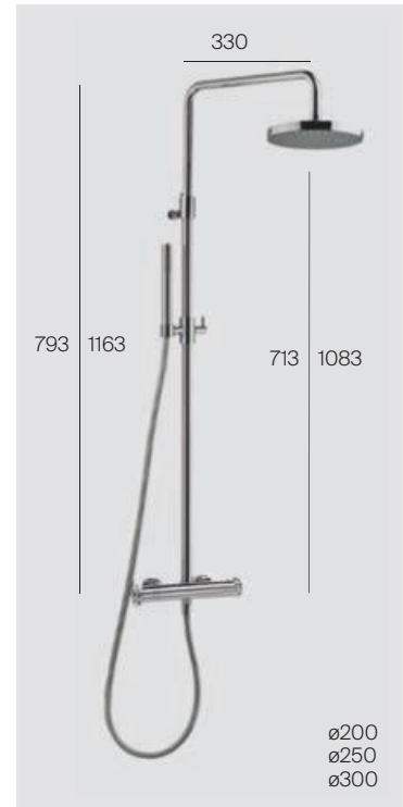
FR389 Columna telescópica termostato 2 duchas Telescopic column thermostatic 2 showers Colonne télescopique thermostatique 2 douches
