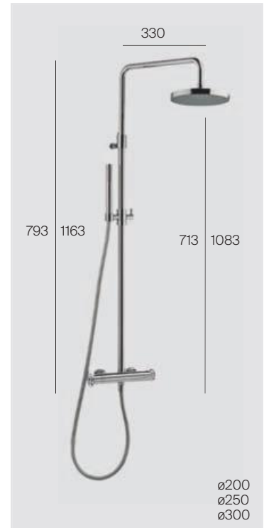
FA389 Columna telescópica termostato 2 duchas Telescopic column thermostatic 2 showers Colonne télescopique thermostatique 2 douches
